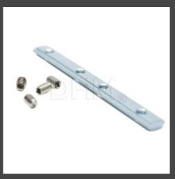
Package contains: 1 xLong pre-assembly nut with holesM5 -5 Series This nut is suitable for use with extruded aluminum profiles. It can be used with 5-series profiles such as 20x20mm and 20x40mm, which have 6mm slots. They are to be inserted before mounting the profile. Threaded tapped hole that allows you to fix the nut with the respective screw. They are suitable for fixing a linear guide to the profile.
